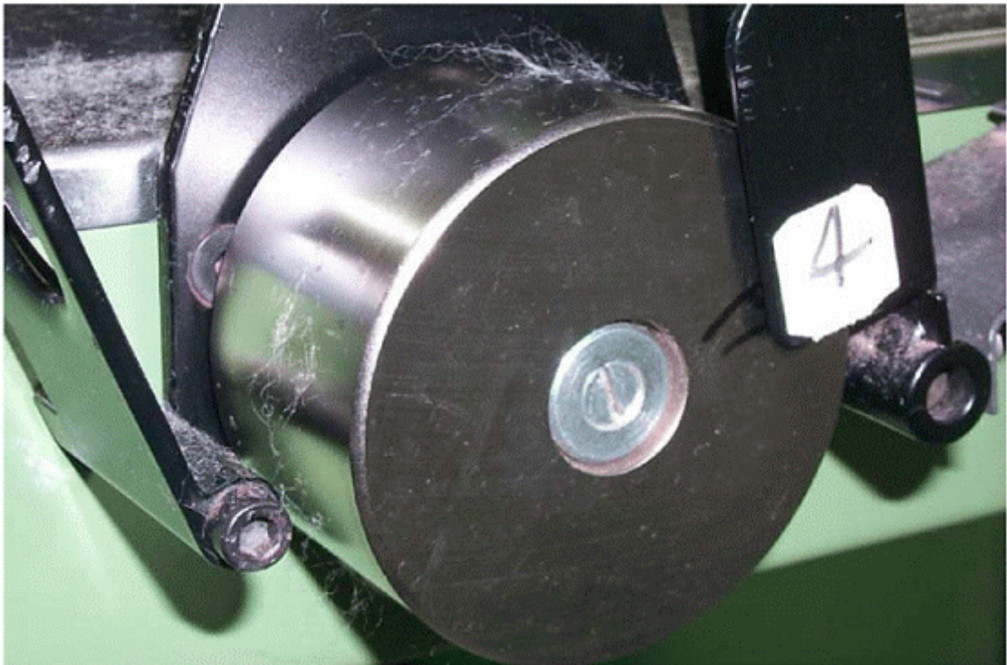
< 2> Sticky deposits on the draw frame creel drive rolls.
